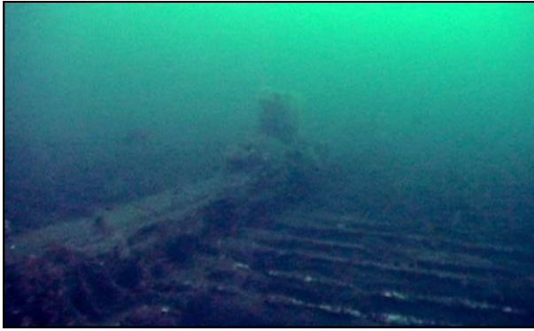
A view of the keelson with ribs perpendicular, stretching out about 15-20 feet on each side.
