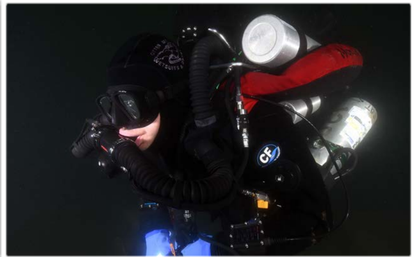
A BOV configured with an inline shut-off valve and access to off-board gas on the diver's left side. The inline shut-off is on the diver's left shoulder.
