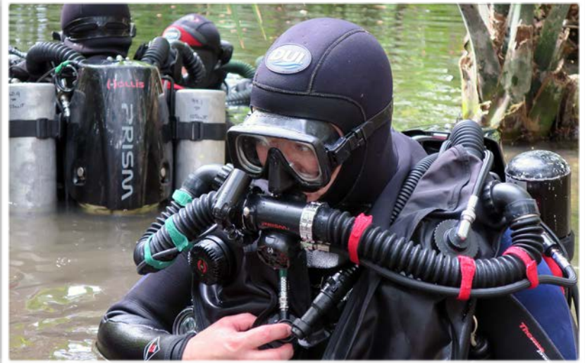
A BOV can be dangerous at the surface when using a hypoxic trimix diluent.
